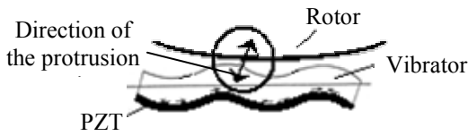
Figure 2. Motion of the protrusion
